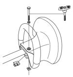
6 Now make a final adjustment to give yourself a comfortable working position. Tighten the screw. CAUTION! The loop handle and hand guard must not be fitted behind the arrow marked on the shaft.
